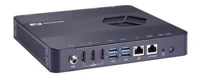
allows users to monitor, manage, and repair remotely. The signage player features one M.2 Key B 3042 for LTE/4G module and one M.2 Key E 2230 for Wi-Fi/Bluetooth; accordingly, it also provides four antenna connectors to establish Wi-Fi or 4G LTE connections. It has four USB 3.1 ports and one LAN for data transmission. The player supports Windows® 10 IoT and can be wall-mounted and VESA mounted as optional requests.
